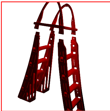
#4: Align the inside/outside rails with deck/handrail.
