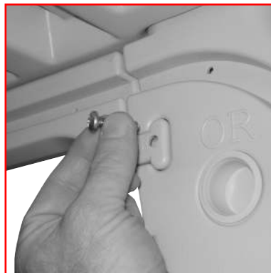
#8: Using the 1/4" - 20 x 1" screws and hex nuts provided attach both outside bridge tabs to the outside ladder rails marked OL & OR. Insert screws through from the inside and fasten with hex nuts on the outside of rail.
