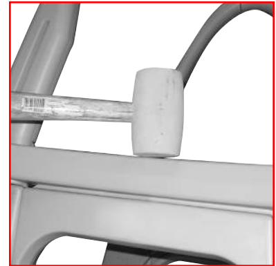
#9: Finish tapping deck all the way down until engaged on to bridge.
