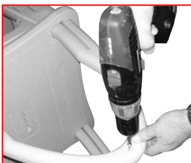
#7: Install right and left ladder bridges.
